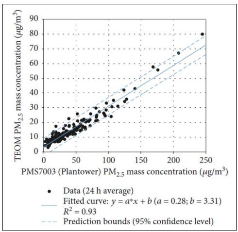
Figure 3-10. Comparison of a Plantower unit (slightly different from but comparable to that used in the PurpleAir) with a TEOM Federal Equivalent Method used for compliance monitoring (Badura et al., 2018). The Plantower is highly correlated, but reads 3.5 times higher than the compliance measurement.
