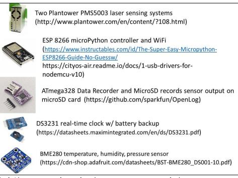
Figure 3-5. PupleAir components that apply a time stamp, measure atmospheric temperature, pressure and relative humidity, store data on an SD card, and provide WiFi interface to the PurpleAir web site.
