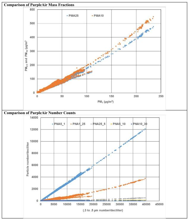
Figure 3-7. Comparison among five collocated PurpleAir sensors for the reported size fractions compared with the smallest size fractions. The manufacturers have apparently included constant multipliers to estimate the different size fractions from the light scattering output of the sensor.
